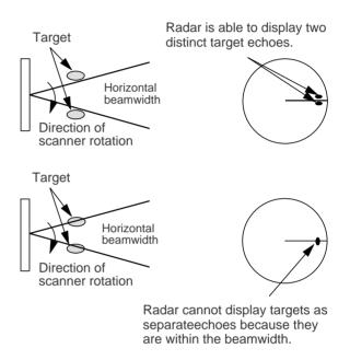
Figure 3-3 Bearing resolution
